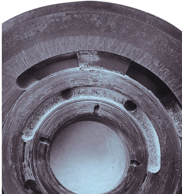
Typical results of wear due to presence of particulate and water contamination.
